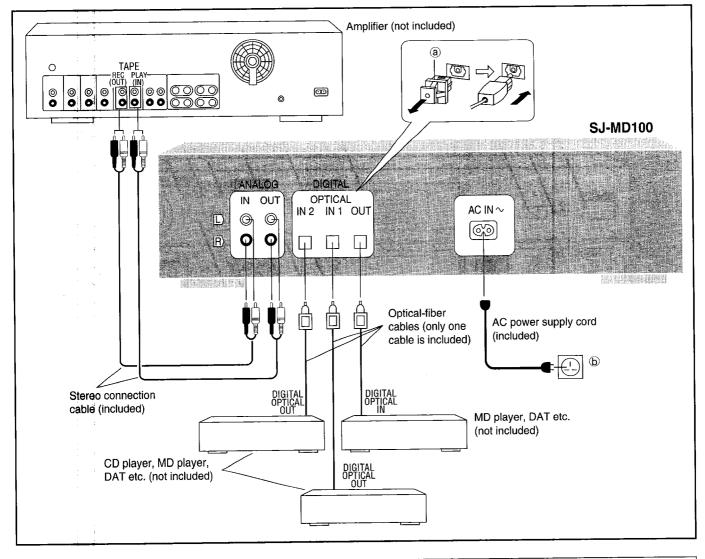
This example shows the unit connected to an amplifier through the ANALOG IN/OUT terminals, and to digital equipment (CD player, MD player, DAT, etc.) through the DIGITAL OPTICAL IN/OUT terminals.
