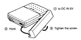
2 Install three size AA (R6) alkaline batteries (not supplied) in the order ① to ③.
